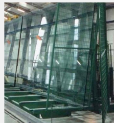
Stacking and Transport Glass sheets are lifted vertically using suction cups with a thin layer of interleaving lucite powder between each sheet for protection against scratches. These are then safely transported in special vans.
