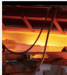
2. Melting and refining Heated in a furnace at around 1600^\circ\text{C} to form molten glass. Refining cools glass and helps remove air bubbles.
